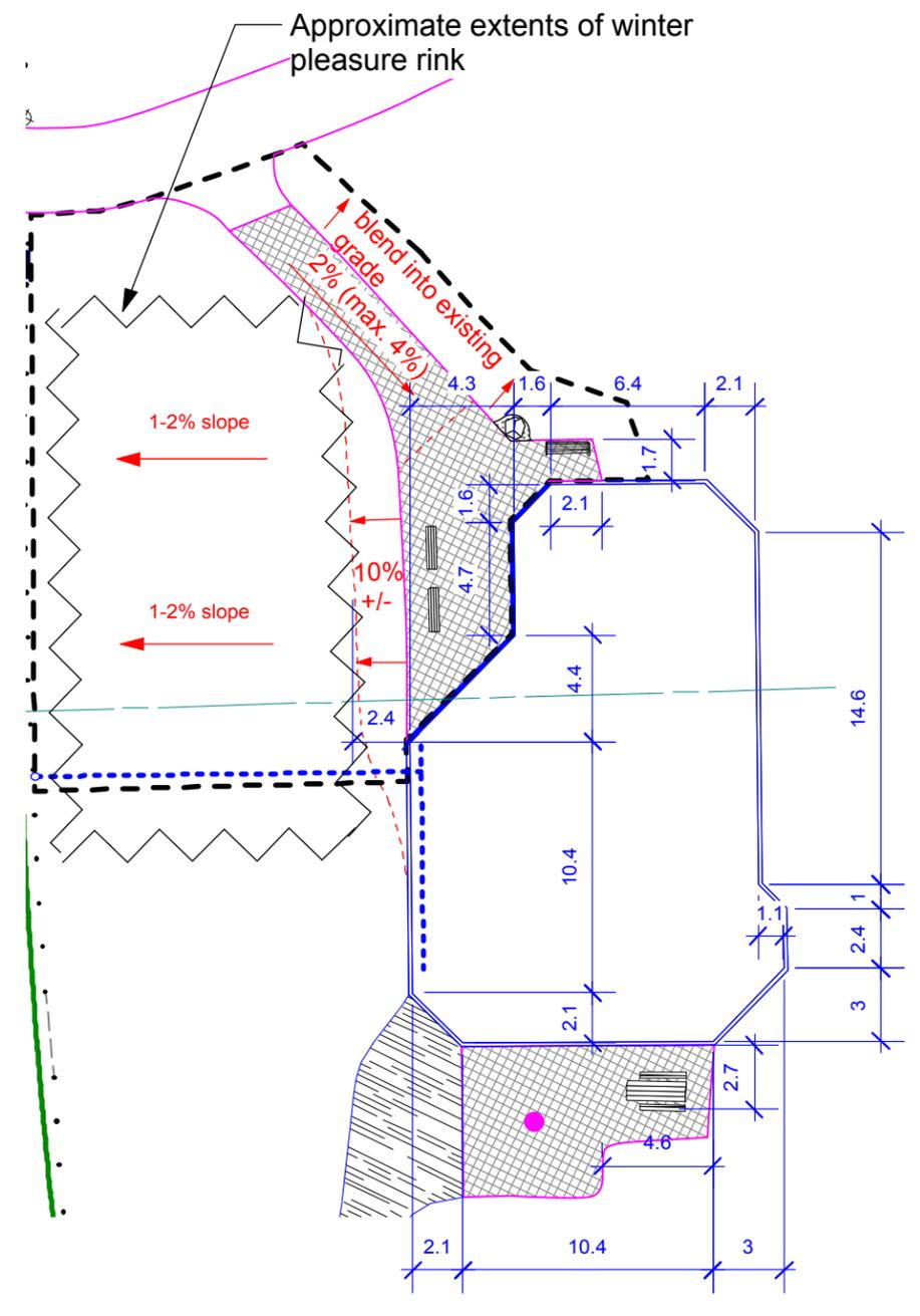
\* All dimensions are in meters and are to inside edge of timber edging.
