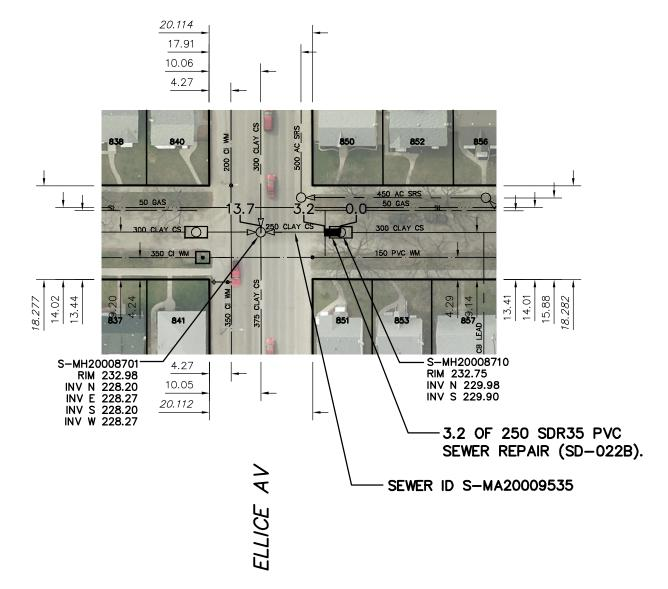
SEWER JUNCTION INFORMATION FROM SEWER VIDEO INSPECTION SEWER ID S-MA20009535 DISTANCE FROM MH ID S-MH20008710 DISTANCE DIAMETER CLOCK \*NO JUNCTIONS\*
