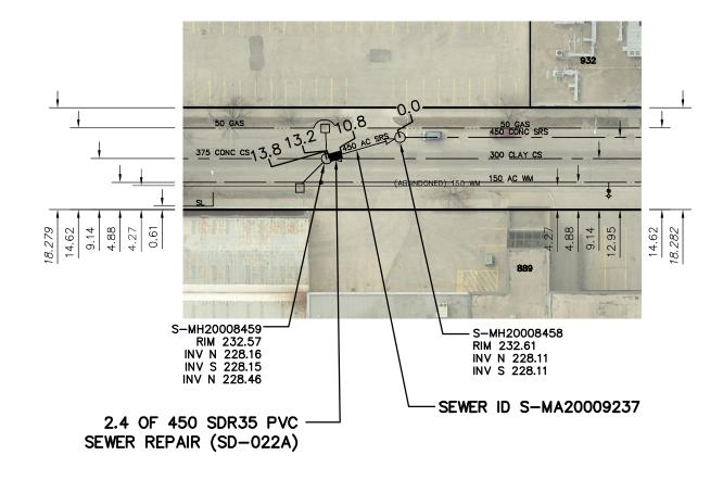
SEWER JUNCTION INFORMATION FROM SEWER VIDEO INSPECTION SEWER ID S-MA20009237 DISTANCE FROM MH ID S-MH20008458 DISTANCE DIAMETER CLOCK \*NO JUNCTIONS\*
