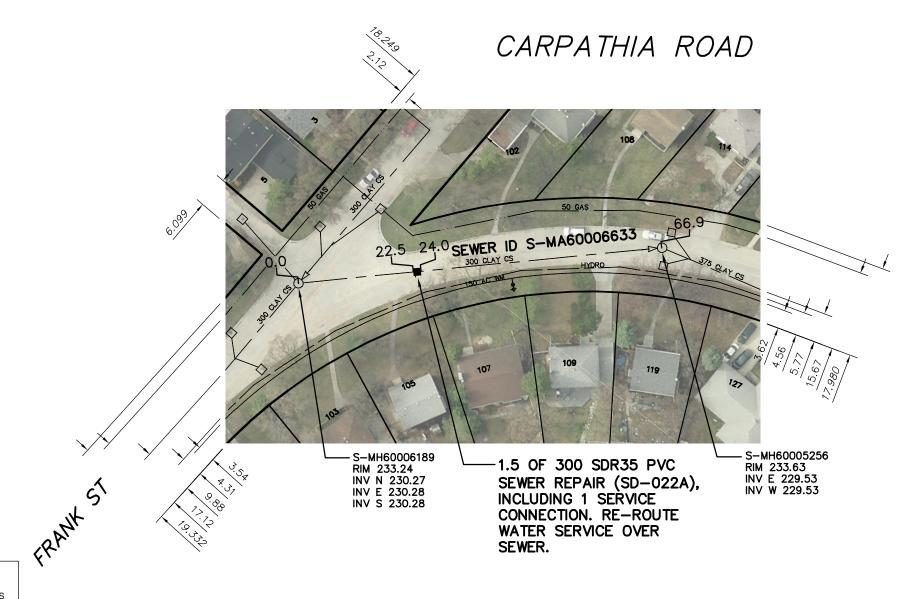
SEWER JUNCTION INFORMATION FROM SEWER VIDEO INSPECTION SEWER ID S-MA60006633 DISTANCE FROM MH ID S-MH60006189 DIAMETER DISTANCE CLOCK 8.8 150 10 9.5 150 22.8 150 41.5 150 10 42.2 150 150 43.8 60.1 150 62.4 150
