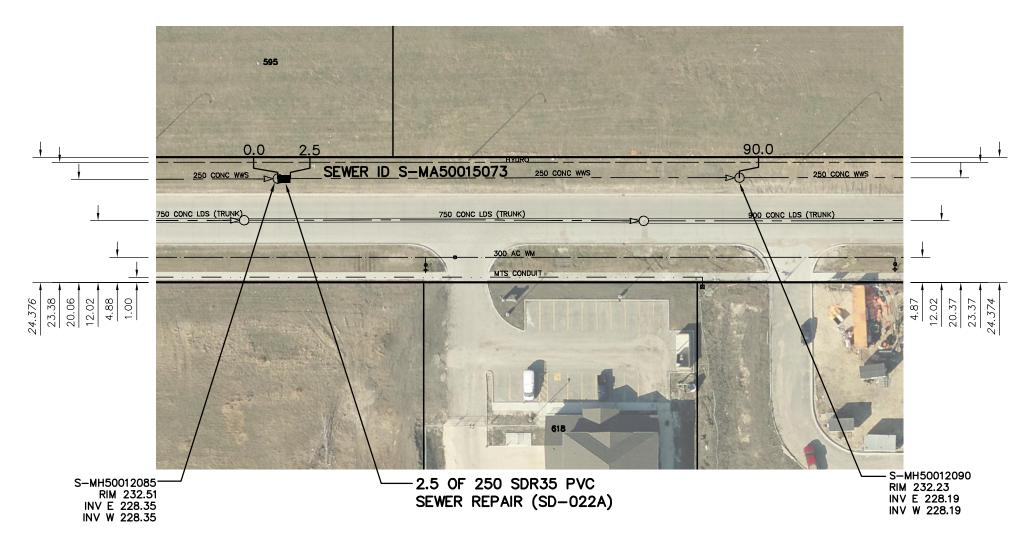
SEWER JUNCTION INFORMATION FROM SEWER VIDEO INSPECTION SEWER ID S-MA50015073 DISTANCE FROM MH ID S-MH50012085 DISTANCE DIAMETER CLOCK 55.3 150
