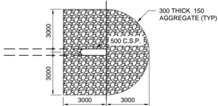
**TYPICAL CULVERT END PROTECTION**
