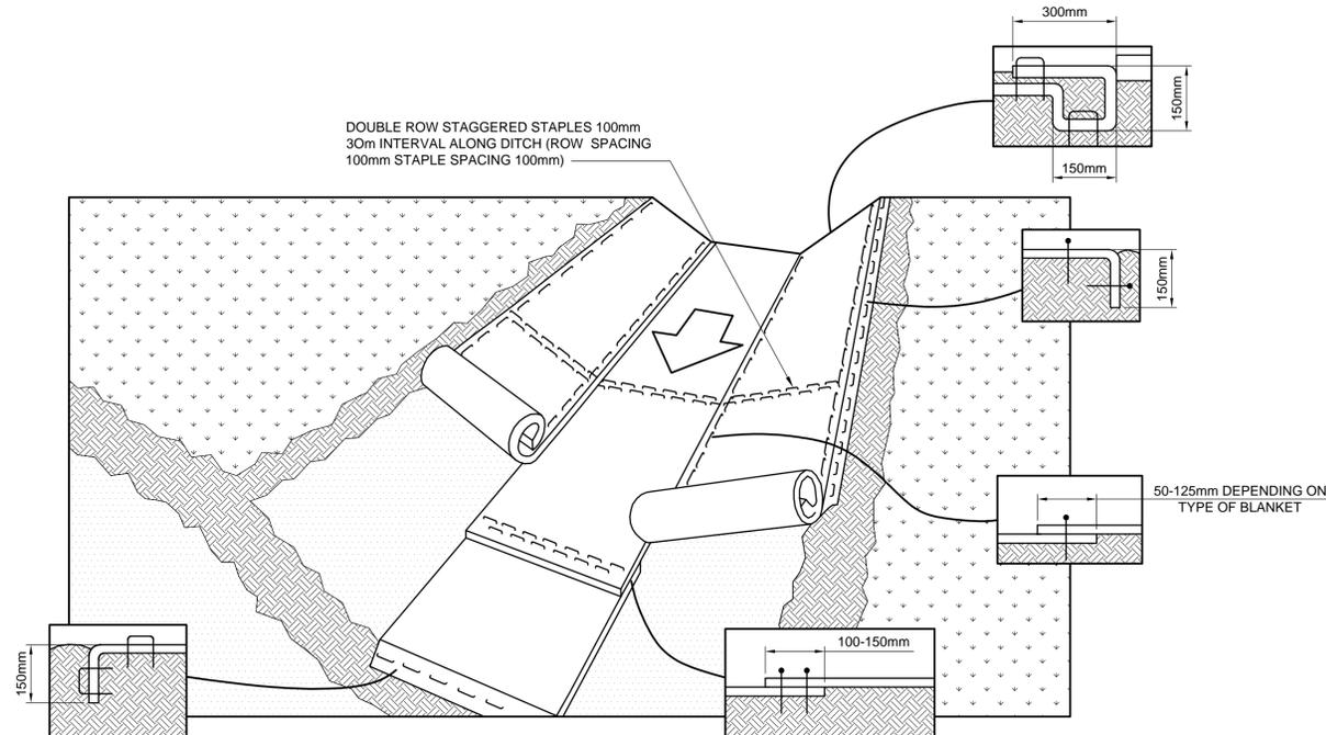
**TYPICAL DRAINAGE CHANNEL INSTALLATION**
