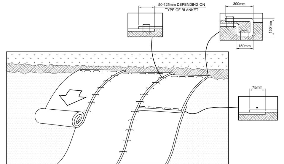
**TYPICAL SLOPE INSTALLATION**
