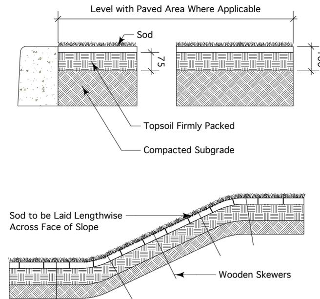
In Every Second Row on Slope and at the Base of the Slope Each Piece of Sod to be Pegged with Two Minimum 250mm Long Wooden Skewers Driven in Below Lawn Level, On Slope 1:2 or Steeper, Each Piece of Sod in Every Row Shall be Pegged
