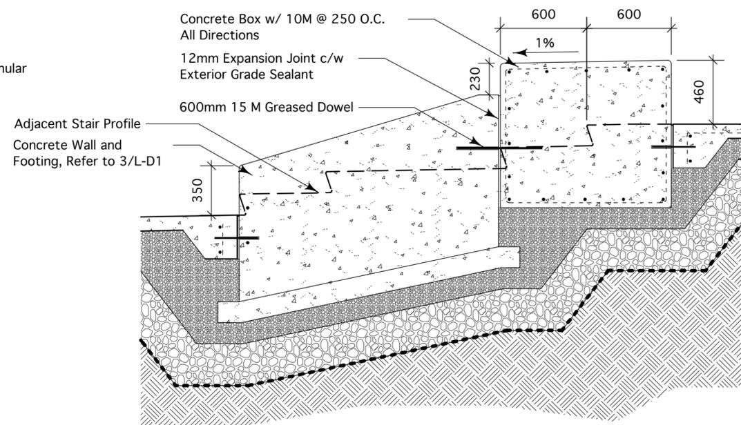
4 Concrete Cheek Wall Type Two & Concrete Box
