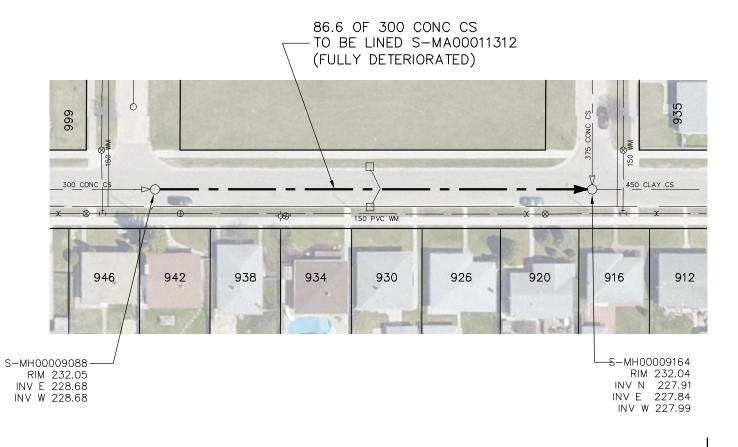
SEWER JUNCTION INFORMATION FROM SEWER VIDEO INSPECTION SEWER ID S-MA00011312 DISTANCE FROM MH ID S-MH00009088 DISTANCE DIAMETER CLOCK 8.5 150 20.9 150 34.0 150 34.3 150 46.6 200 10 47.2 200 57.3 150 150 81.2
