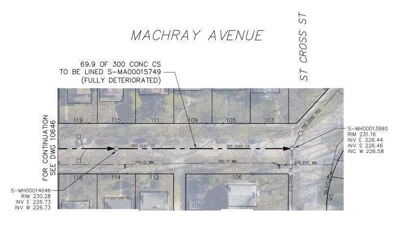
SEWER JUNCTION INFORMATION FROM SEWER VIDEO INSPECTION SEWER ID S-MA00015749 DISTANCE FROM MH ID S-MH00014046 DISTANCE DIAMETER CLOCK 6.2 150 6.8 150 21.4 150 10 22.0 150 36.7 150 10 37.3 150 44.3 150 10 150 11 60.0 150
