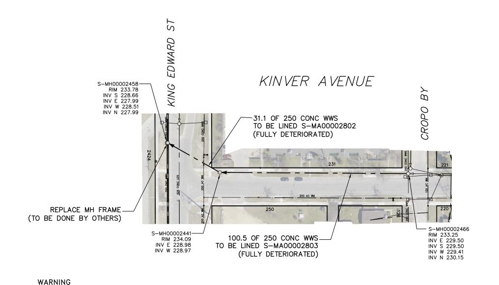
SEWER JUNCTION INFORMATION FROM SEWER VIDEO INSPECTION SEWER ID S-MA00002803 DISTANCE FROM MH ID S-MH00002466 DIAMETER DISTANCE CLOCK 68.4 150 11 86.8 150 12
