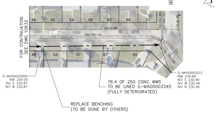
SEWER JUNCTION INFORMATION FROM SEWER VIDEO INSPECTION SEWER ID S-MA00003345 DISTANCE FROM MH ID S-MH00002950 DIAMETER CLOCK DISTANCE 11.5 150 9 12.1 150 26.0 150 10 27.5 150 30.7 150 10 37.6 150 10 44.3 150 53.9 200 12 59.7 150 150 66.7
