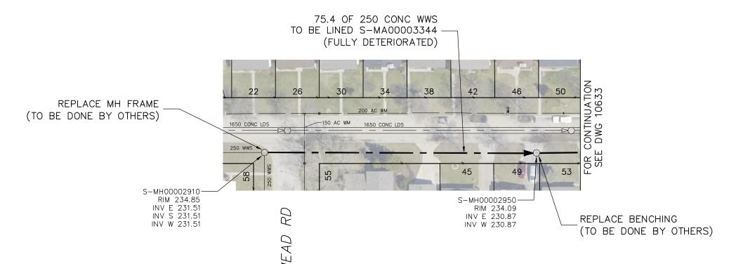
SEWER JUNCTION INFORMATION FROM SEWER VIDEO INSPECTION SEWER ID S-MA00003344 DISTANCE FROM MH ID S-MH00002910 DISTANCE DIAMETER CLOCK 10 12.8 150 10 18.5 10 150 22.4 150 32.6 10 38.7 150 45.5 150 54.6 150 9 55.8 150 71.1 150 10 71.6
