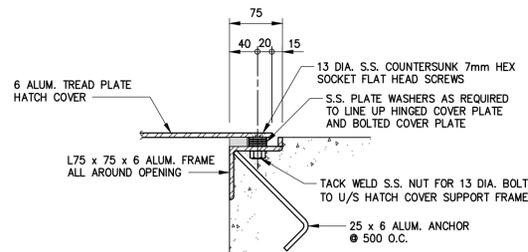
HATCH COVER BOLT-DOWN SECTION (F-S7/S6)
