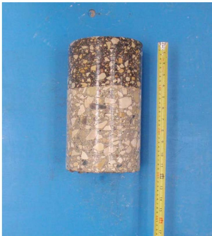
Core sample from Testhole TH04
