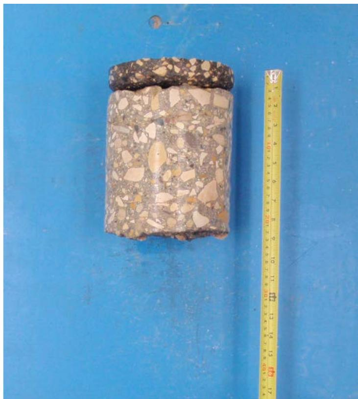
Core sample from Testhole TH12
