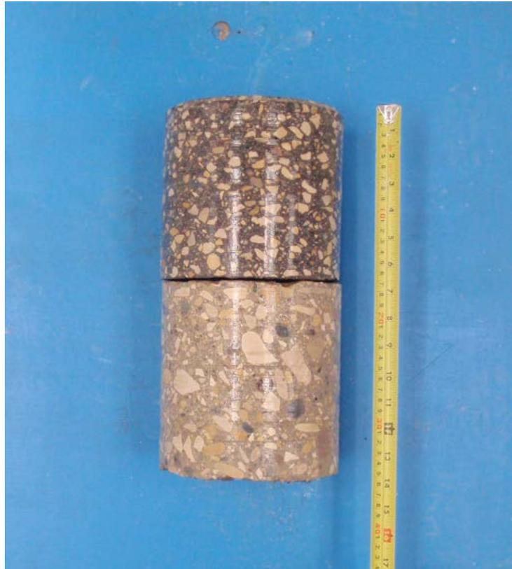
Core sample from Testhole TH07
