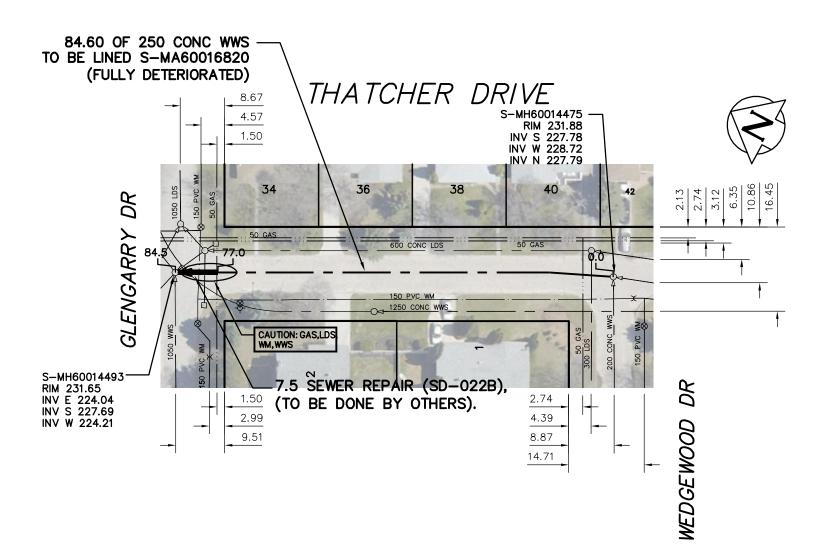
SEWER JUNCTION INFORMATION FROM SEWER VIDEO INSPECTION SEWER ID S-MA60016820 DISTANCE FROM MH ID S-MH60014475 DISTANCE DIAMETER CLOCK 13.5 150 30.0 150 49.5 150 67.2 150
