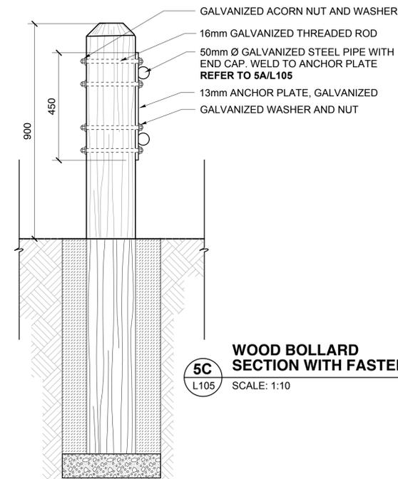
**5C WOOD BOLLARD SECTION WITH FASTENERS**
