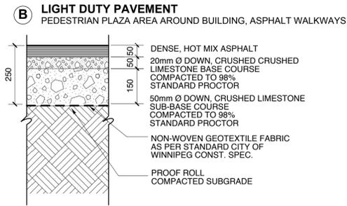
**1 ASPHALT PAVEMENT SECTIONS**
