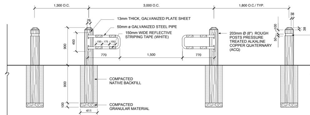
**NOTE:** FOR TWO POSTS ADJACENT TO REFLECTIVE ARMATURES PROVIDE 13mm DEEP REVEAL FOR REFLECTIVE TAPE. APPLY REFLECTIVE TAPE IN GROOVE BEFORE INSTALLING IN GROUND. REFLECTIVE TAPE: 3M SCOTCHLITE DIAMOND GRADE SERIES 981, WHITE OR APPROVED EQUAL
