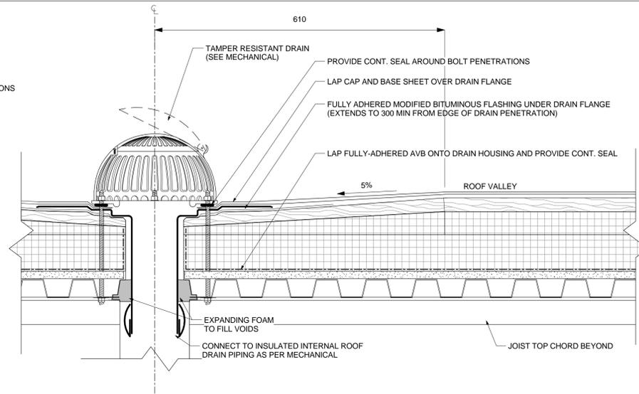
2 ROOF SECTION DETAIL - DRAIN
