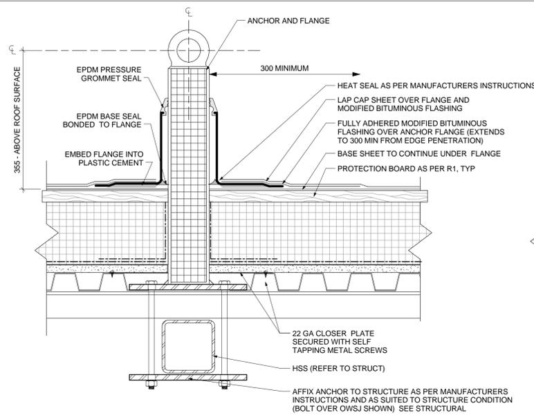
1 ROOF SECTION DETAIL - ROOF ANCHOR
