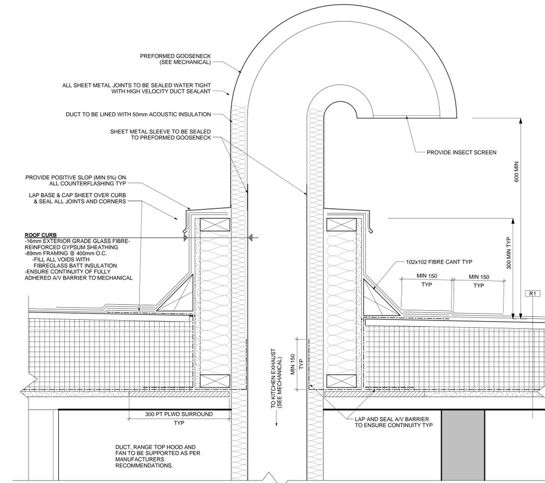
7 ROOF SECTION DETAIL - KITCHEN EXHAUST
