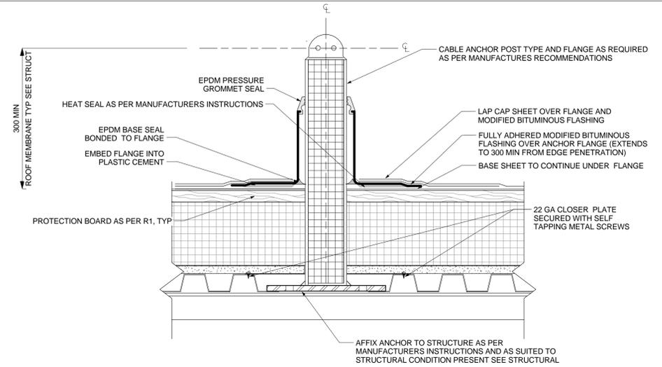
3 ROOF SECTION DETAIL - FALL ARREST CABLE ANCHOR
