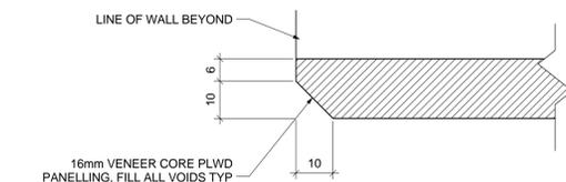
14 TYPICAL PLWD CHAMFER DETAIL
