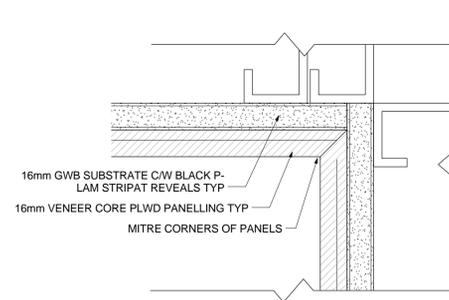
18 TYPICAL INSIDE CORNER PLAN DETAIL @ PLWD PANELLING
