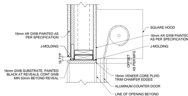
13 TYPICAL PLAN DETAIL @ COUNTER DOOR HEAD
