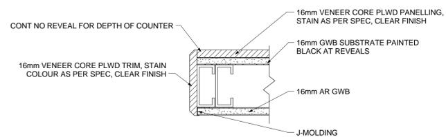
8 TYPICAL PLAN DETAIL @ COUNTER DOOR JAMB
