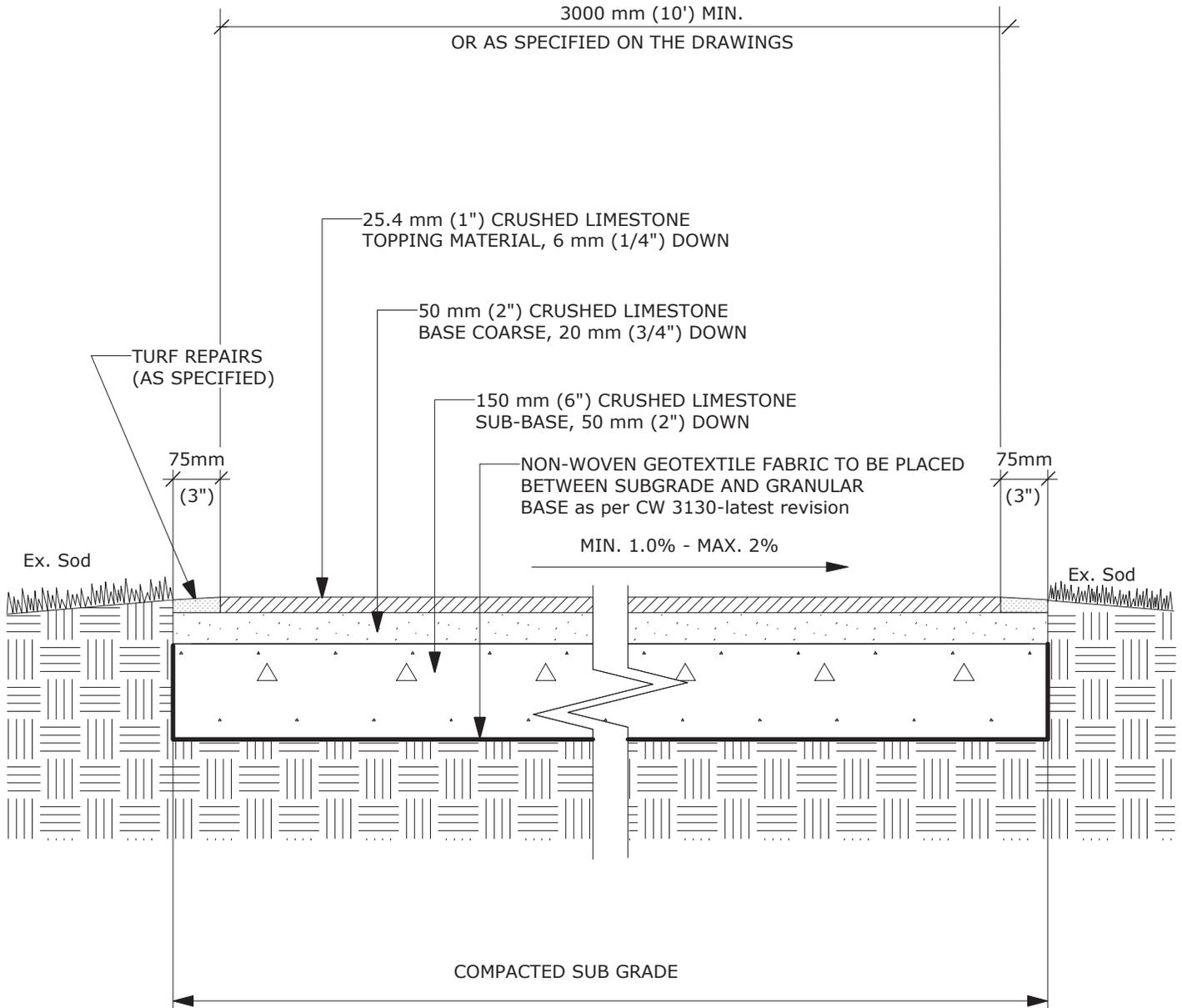
DIMENSIONS SHOWN ARE IN MILLIMETRES UNLESS OTHERWISE SPECIFIED
