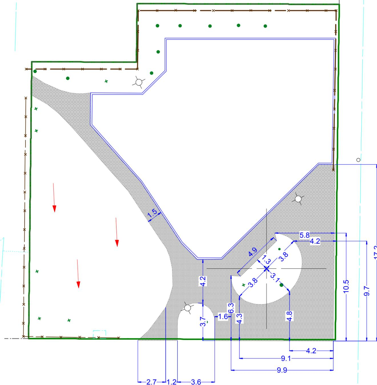
\* NOTE: All dimensions are in Meters and all dimensions are to the outside of the timber edging.
