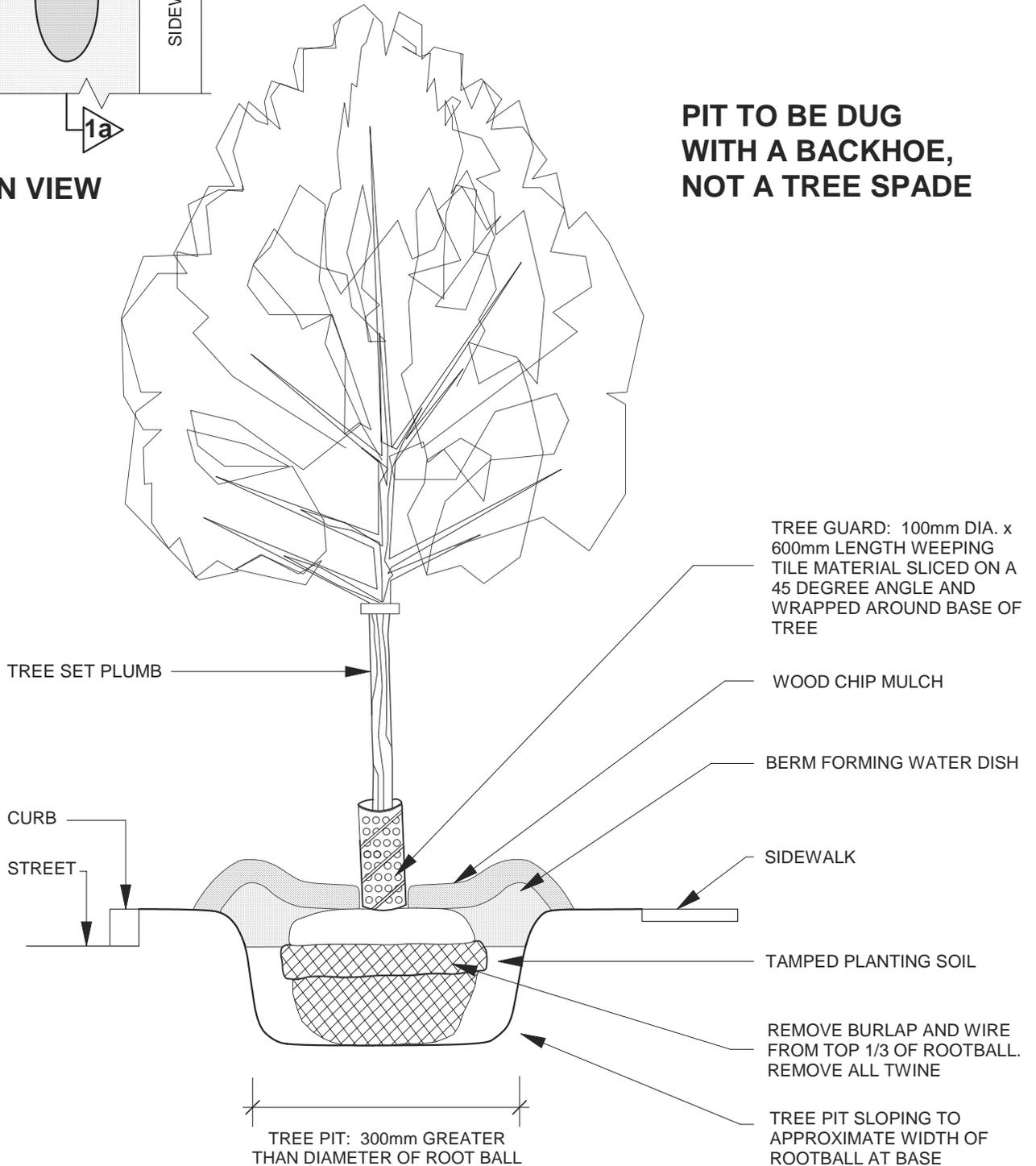
TREE GUARD: 100mm DIA. x 600mm LENGTH WEAVING TILE MATERIAL SLICED ON A 45 DEGREE ANGLE AND WRAPPED AROUND BASE OF TREE
