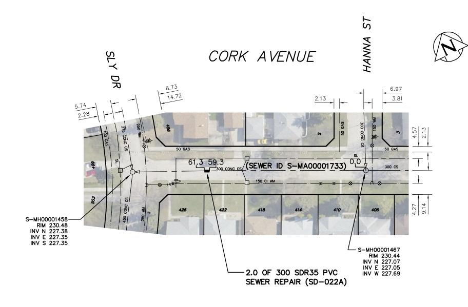
SEWER JUNCTION INFORMATION FROM SEWER VIDEO INSPECTION SEWER ID S-MA00001733 DISTANCE FROM MH ID S-MH00001467 DISTANCE DIAMETER CLOCK 10 13.2 150 10 27.5 150 10 40.1 150 10 43.7 150 11 150 45.5 55.7 150 10 67.7 150 10
