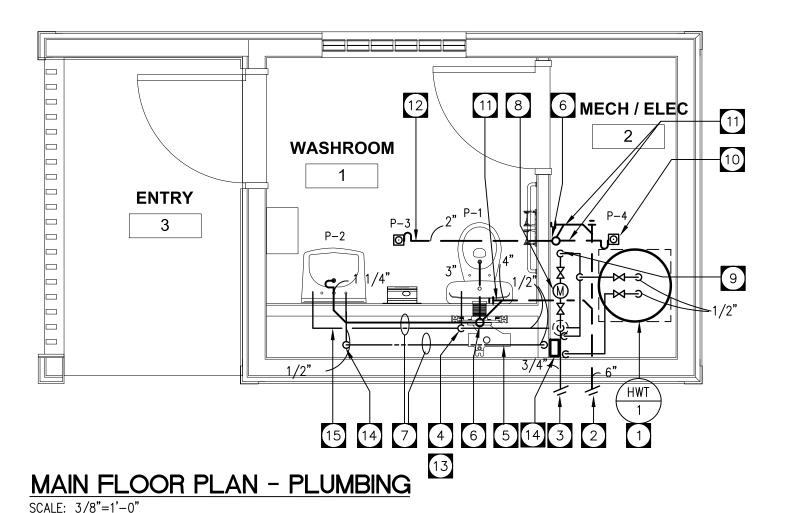
RUN SANITARY DRAINAGE PIPING & DOMESTIC HOT & COLD WATER LINES WITHIN FURRED OUT WALL CAVITY TO SERVE WASHROOM LAVATORY &
