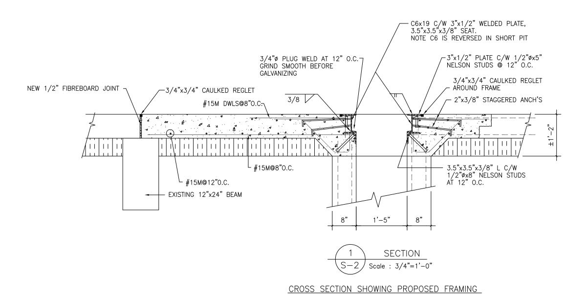
Scale : 3/4" = 1'-0" NOTE: ALL STEEL MEMBERS & ANCHORS TO BE HOT DIP GALVANIZED
