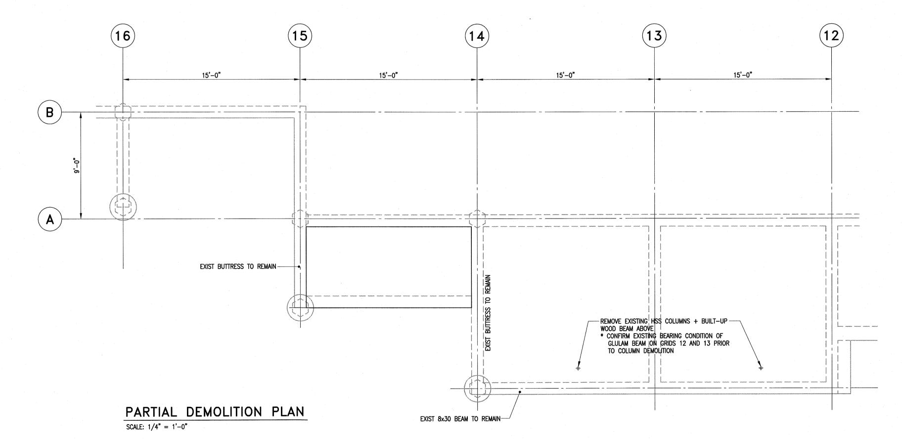
REMOVE HSS POSTS AND BUILT UP 2x8 WOOD BEAM AROUND TOP OF EXISTING CURTAIN WALL — SITE CONFIRM WITH CONTRACT ADMINISTRATOR PRIOR TO DEMOLITION. CUT COLUMNS OFF AND PATCH SLAB SURFACE AS REQUIRED. DO NOT DAMAGE REMAINDER OF EXISTING FINISHES. CONFIRM CONDITION AND EXISTING DETAILS WITH RESPECT TO ROOF FRAMING ABOVE PRIOR TO DEMOLITION.
