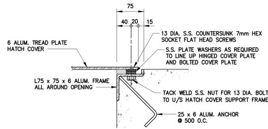
**HATCH COVER BOLT-DOWN SECTION** (F-S6/S5)
