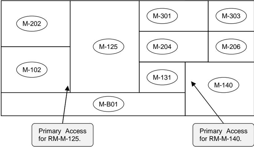
**Figure 3-3 : Multi-Level Room Examples – Elevation View**
