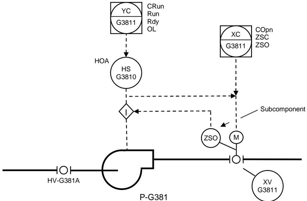
**Figure 7-2 : Subcomponents – Mechanical and Process Equipment**
