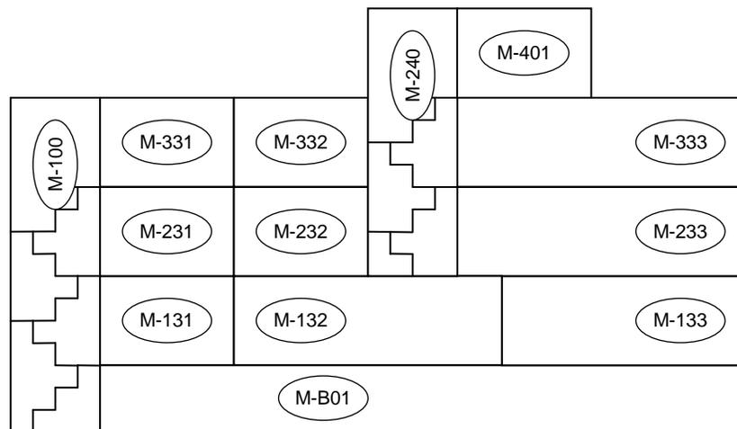
**Figure 3-2 : Stairwell Identification Examples – Elevation View**
