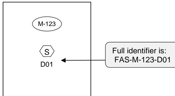
**Figure 6-3 : Room Numbering on Drawings – Plan View**
