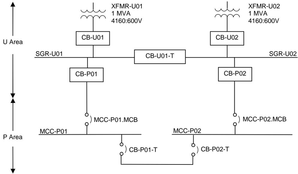
**Figure 6-1 : Sample Tie Breaker Identification**
