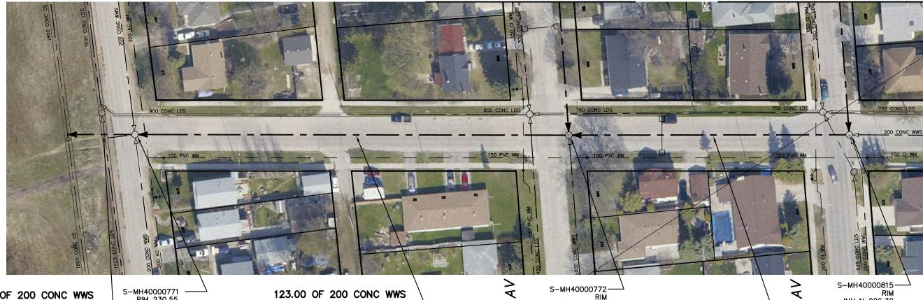
19.80 OF 200 CONC WWS TO BE LINED S-MA70021186 (FULLY DETERIORATED)
