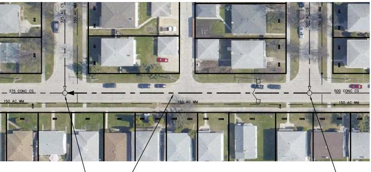
SEWER JUNCTION INFORMATION FROM SEWER VIDEO INSPECTION SEWER ID S-MA40010381 DISTANCE FROM MH ID S-MH40009469 DISTANCE DIAMETER CLOCK 4.8 10 12.4 150 10 10 23.3 150 24.1 150 2 31.0 150 10 44.1 150 10 100 11 56.4 150 68.0 10 80.3 150 10 92.6 150 11
