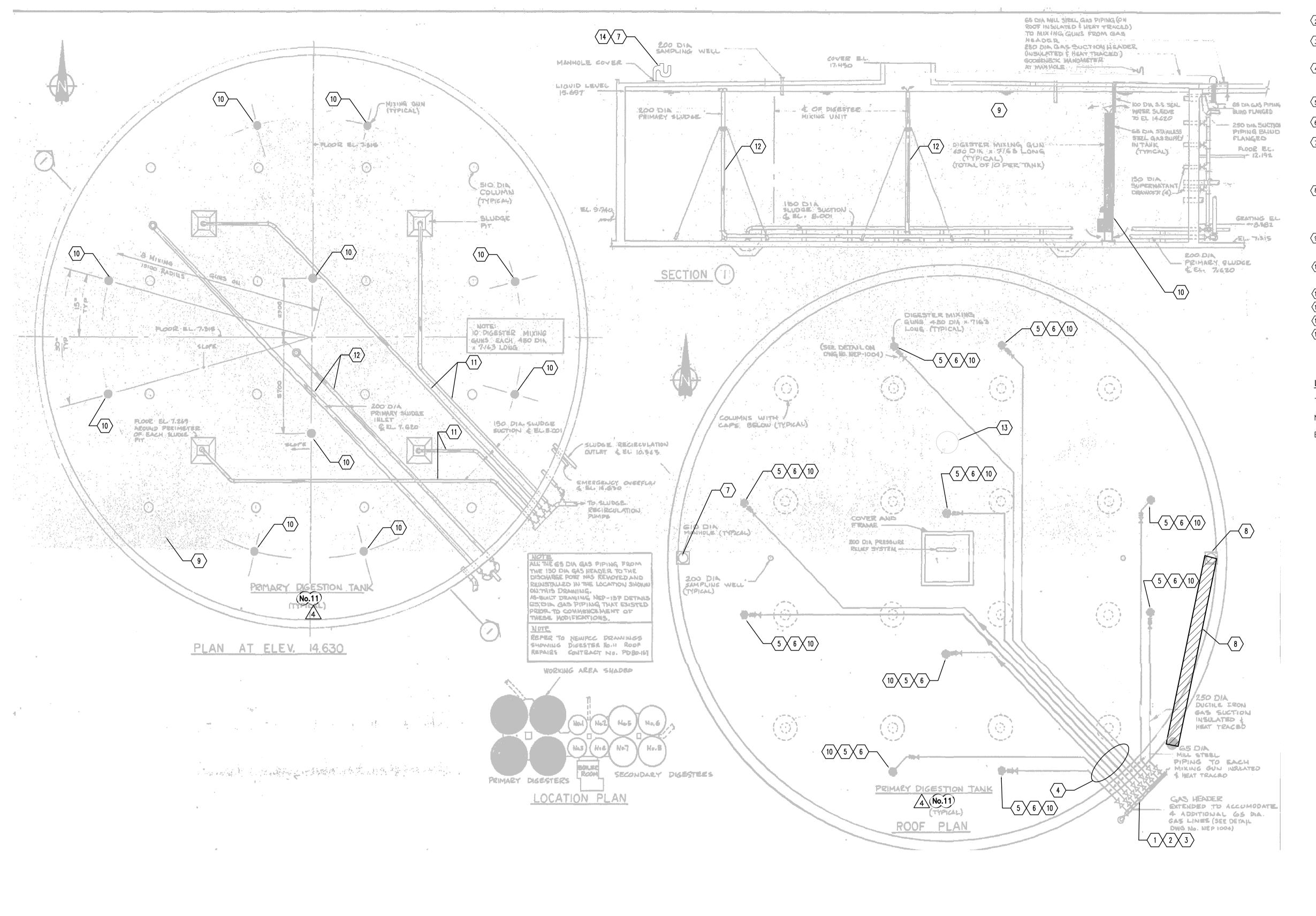
1 DISCONNECT HEAT TRACING. DEMOLISH AND REMOVE MIXING GAS SUPPLY PIPING, HEAT TRACING, INSULATION AND VENT PIPING PENETRATING THROUGH ROOF OF DIGESTER GALLERY.
