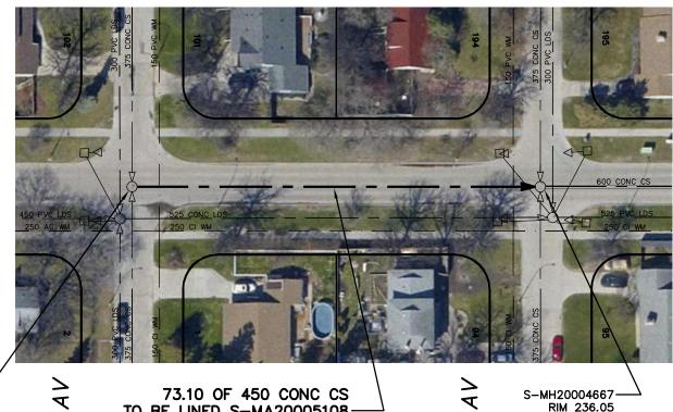
SEWER JUNCTION INFORMATION FROM SEWER VIDEO INSPECTION SEWER ID S-MA20005108
