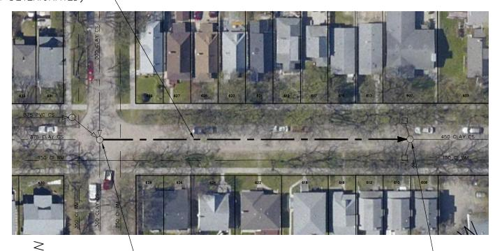
SEWER JUNCTION INFORMATION FROM SEWER VIDEO INSPECTION SEWER ID S-MA60009075 DISTANCE FROM MH ID S-MH60007479 DISTANCE DIAMETER CLOCK 16.4 150 17.0 150 28.1 150 31.3 150 31.9 150 11 46.8 150 47.5 150 61.7 150 62.3 150 72.3 150 78.4 150 11 84.6 150 85.3 150 10
