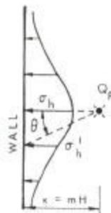
Figure 25.5: Horizontal pressures on a wall due to point and line load surcharges.
