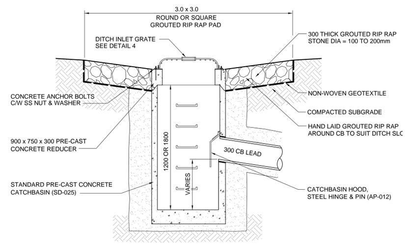
3 DITCH INLET DETAIL IN SECTION
