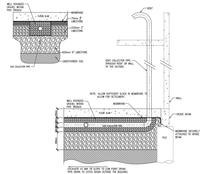
**DETAIL - MODIFIED METHANE GAS PIPING INSTALLATION**
