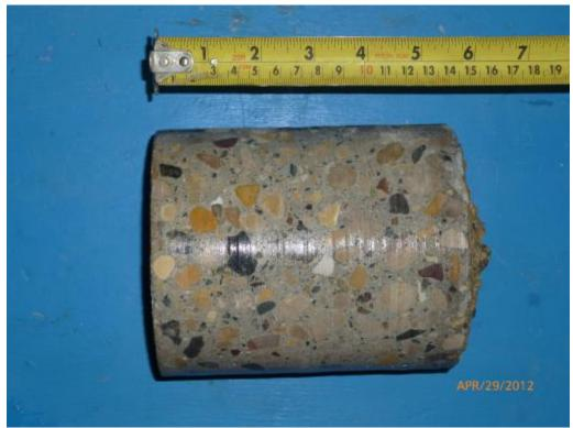
Figure 6 – Core sample obtained from concrete slab
