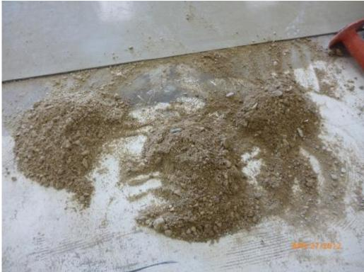
Figure 3 – Granular base obtained from test hole
