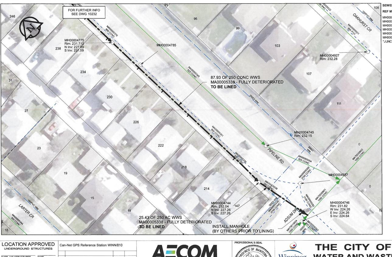
**SEWER JUNCTION INFORMATION** CLOCK AT SIZE\* MH00004775 15.8 150Ø MH00004775 30.3 150Ø 01 MH00004775 45.6 150Ø 02 MH00004775 150Ø MH00004775 73 150Ø MH00004775 86.3 150Ø 01 \*JUNCTION INFORMATION FROM VIDEO INSPECTION
