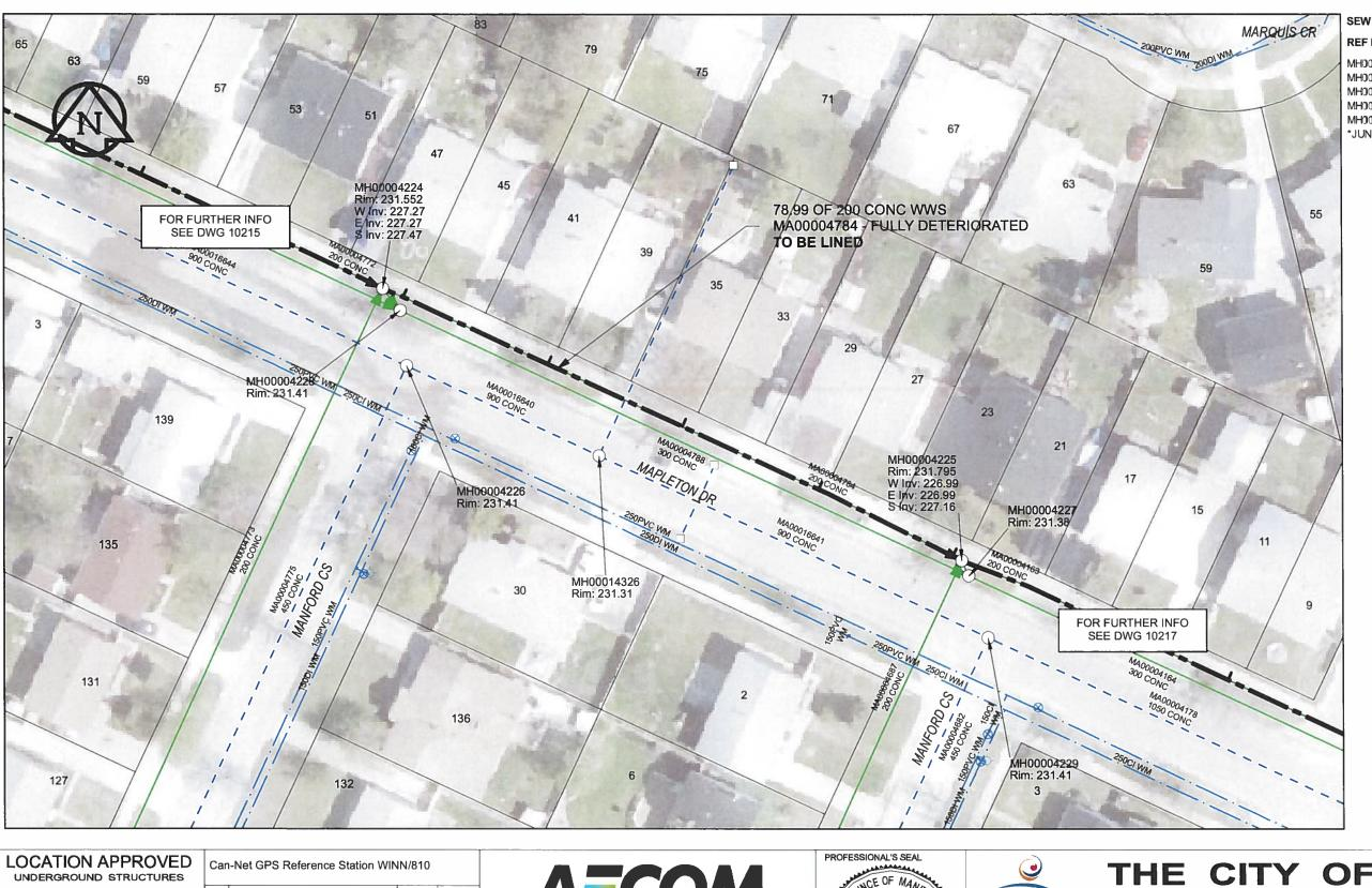
SEWER JUNCTION INFORMATION DIST FROM REF MH\* CLOCK AT\* SIZE\* **REF MH** MH00004224 150Ø 2.7 MH00004224 150Ø 22.4 10 MH00004224 40.7 150Ø 10 MH00004224 59.2 150Ø 10 77.7 MH00004224 150Ø 10 \*JUNCTION INFORMATION FROM VIDEO INSPECTION
