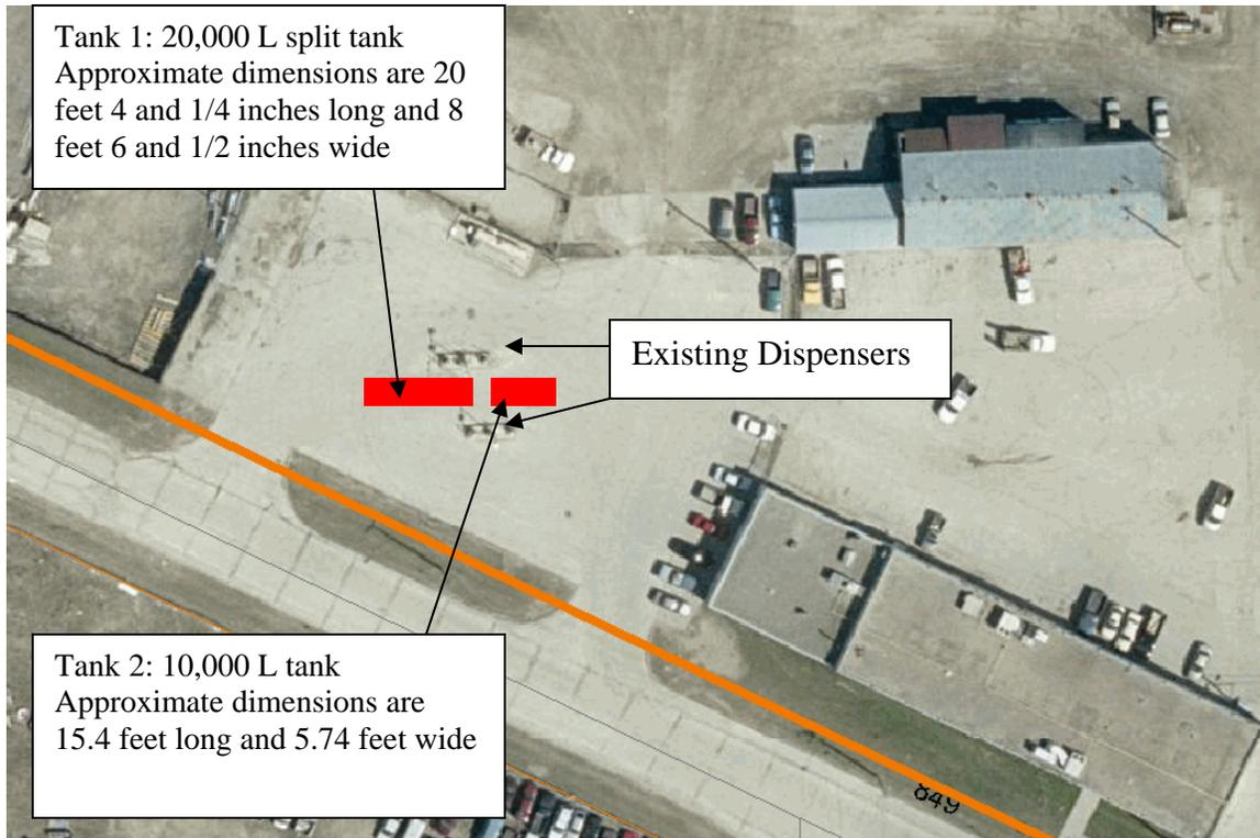
Note: Dimensions are approximate only and depend on the size of tank bid. The Bidder is required to take actual measurements for bidding purposes. Should the tank size measurement deviate from the attached, it is the Contractors responsibility to ensure it will meet regulatory compliance.
