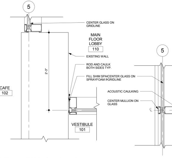
6 DETAIL @ EXISTING WALL AND CURTAINWALL
