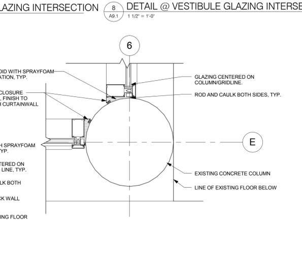
12 DETAIL @ EXISTING COLUMN AND CURTAINWALL
