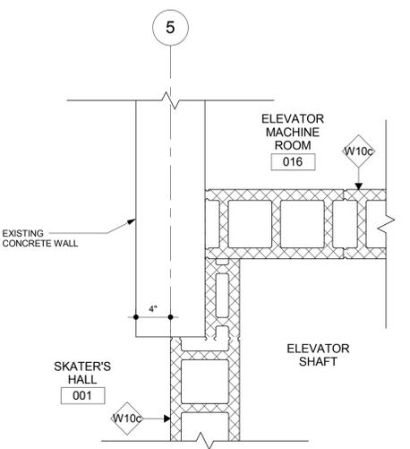
4 DETAIL @ ELEVATOR SHAFT & EXIST. CONCRETE WALL
