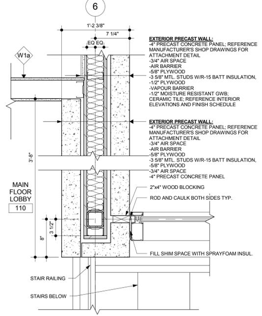
3 DETAIL @ PRECAST AND CURTAINWALL
