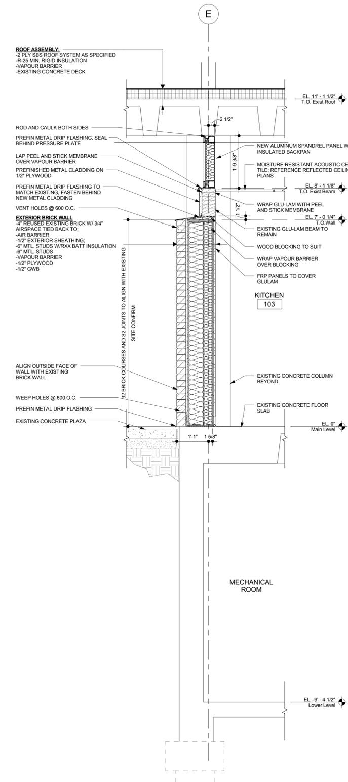
4 WALL SECTION @ NEW BRICK WALL
