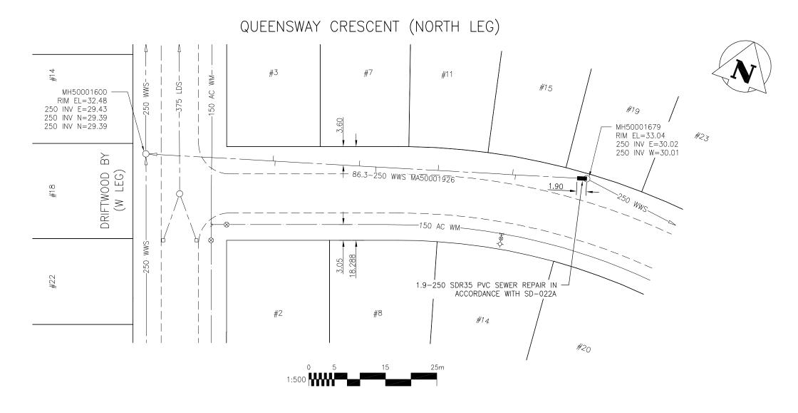
SEWER JUNCTION INFORMATION FOR SEWER ID MA50001926 REFERENCE-METERS WEST OF MANHOLE MH50001679
