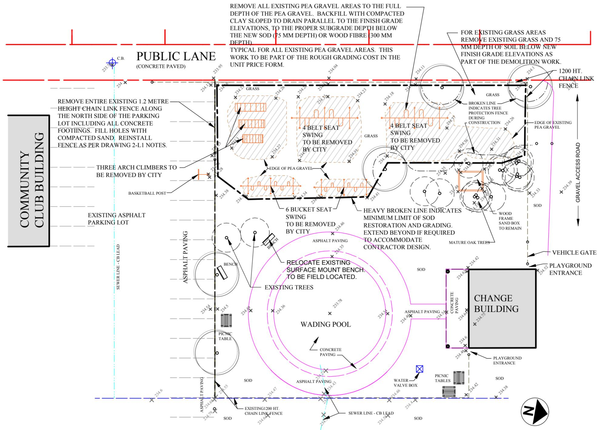
REMOVE ALL EXISTING PEA GRAVEL AREAS TO THE FULL DEPTH OF THE PEA GRAVEL. BACKFILL WITH COMPACTED CLAY SLOPED TO DRAIN PARALLEL TO THE FINISH GRADE ELEVATIONS, TO THE PROPER SUBGRADE DEPTH BELOW THE NEW SOD (75 MM DEPTH) OR WOOD FIBRE (300 MM DEPTH). TYPICAL FOR ALL EXISTING PEA GRAVEL AREAS. THIS WORK TO BE PART OF THE ROUGH GRADING COST IN THE UNIT PRICE FORM.
