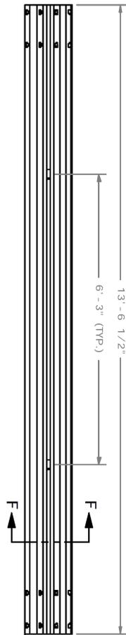
12'-6" W-Beam Section, 12 gauge
