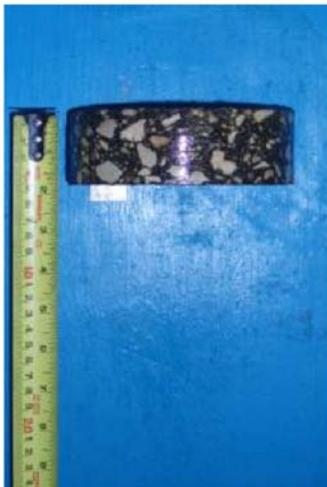
**Core sample from Testhole TH20**
