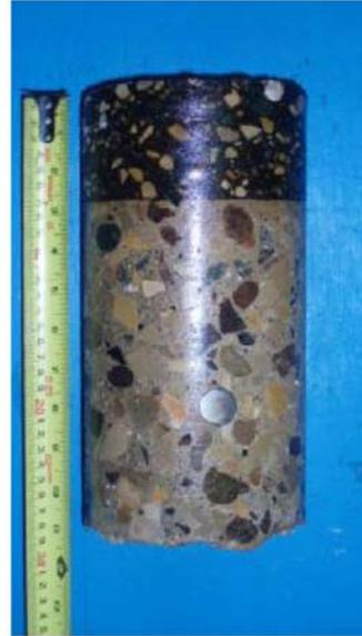
Core sample from Testhole TH7
