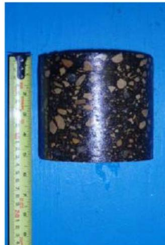
**Core sample from Testhole TH17**
