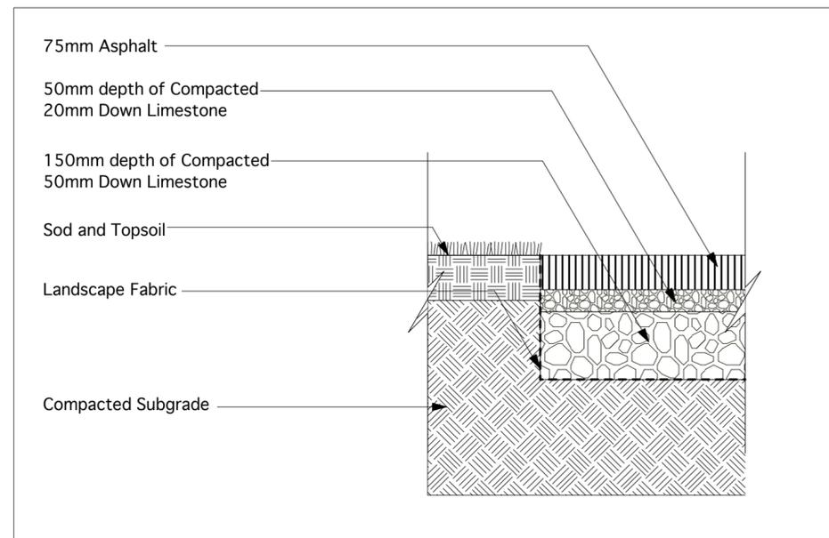
4 Elwick Asphalt Paving Detail
