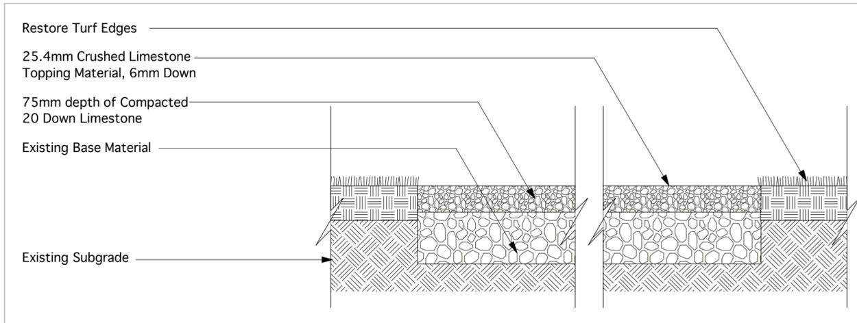
3 Granular Surfacing Detail
