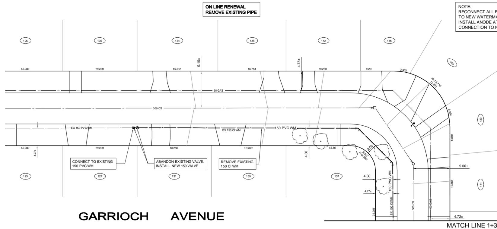
NOTE: RECONNECT ALL EXISTING COPPER SERVICES TO NEW WATERMAIN. INSTALL ANODE AT EVERY COPPER WATER SERVICE CONNECTION TO NEW PVC WATERMAIN.
