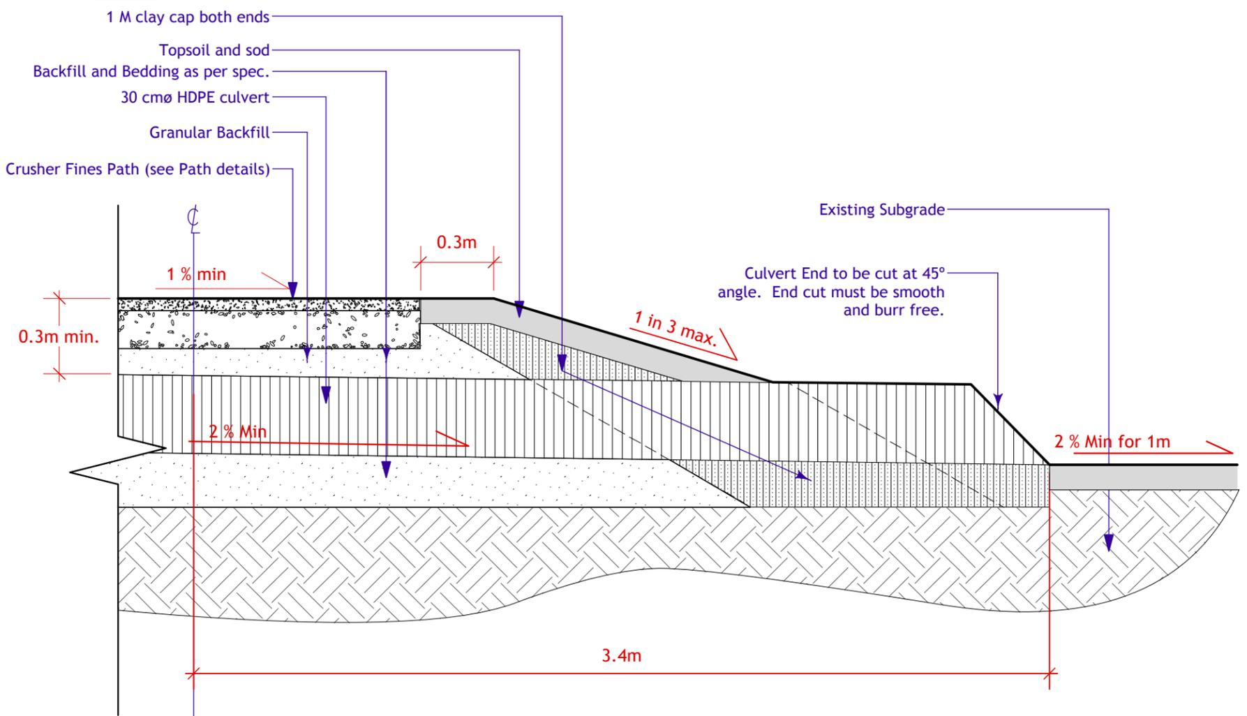
**3 Section through Path and Culvert**
