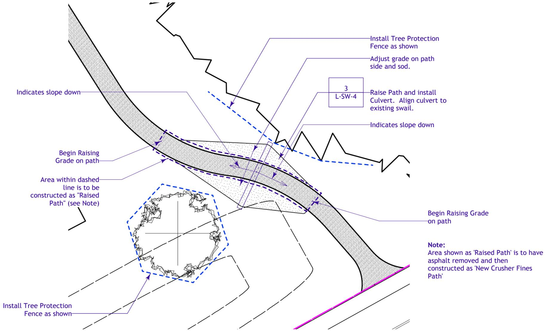
**1** Culvert Area Detail Plan
