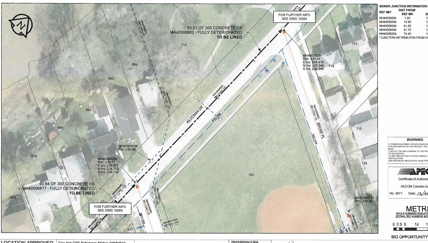
DIST FROM\* REF MH SIZE\* CLOCK AT\* MH40006294 1.20 150Ø 10 MH40006294 15.90 150Ø 10 MH40006294 150Ø 11 MH40006294 51.70 150Ø 01 MH40006294 74.40 150Ø 01 \*JUNCTION INFORMATION FROM VIDEO INSPECTION
